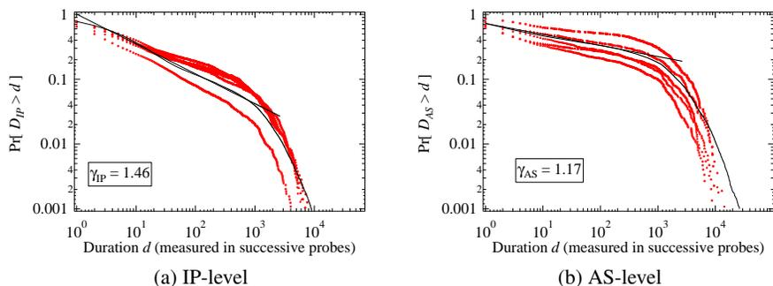
**Figure 3.** The complementary cumulative distribution function of the route duration on log-log scale. The markers represent distributions for five individual source–destination pairs with typical behavior. The measurements are aggregated into a single distribution (solid line) and fitted with  $F(d) = Cd^{1-\gamma}$ . The fit results are presented as the straight lines; the power-law coefficients are found as  $\gamma_{IP} = 1.46$  and  $\gamma_{AS} = 1.17$ .
