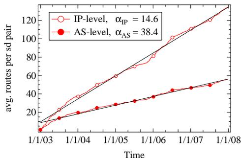
**Figure 2.** The average number of discovered routes between the source–destination pairs at both the AS- and IP-level, counting from January 1, 2003. The measurements have been fitted with a line. The fit at the IP-level resulted in a discovery rate of 14.6 days per route, while at the AS-level the fit provided 38.4 days per route.
